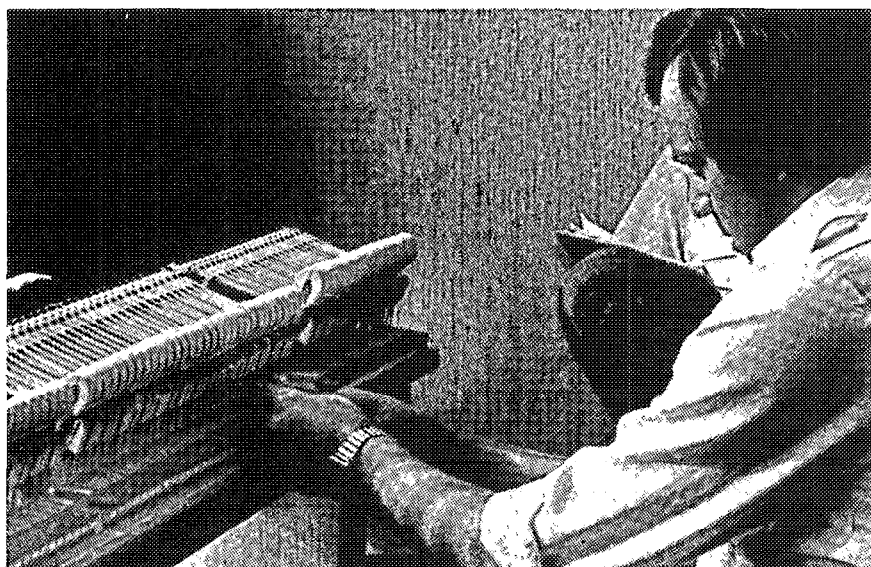
Backcheck regulation. Backchecks should be directly behind hammer tails, evenly spaced and straight up and down.
